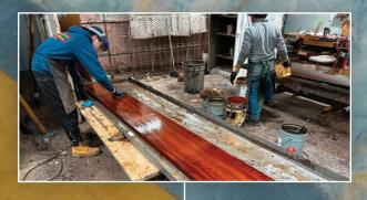
The Basilica pews are stripped of varnish and prepped for extensive sanding and refinishing at Kittinger's facility.
